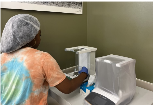
Keiona Williams '24 weighs powdered pumice clasts to analyze on the new ICP-MS instrument.
