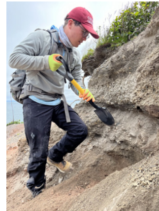
Digging a bench to allow for stable footing when exposing an outcrop.
