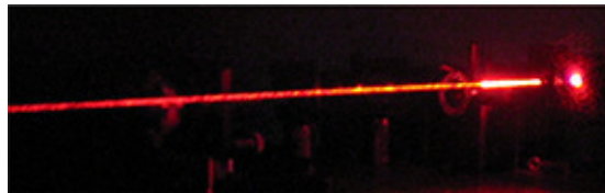
Figure 1.1: A laser beam from a HeNe laser seen due to scattering.
