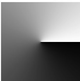
Figure 3.15: Spiral phase encoded in gray scale (white=0, black= 2\pi ) for programming the SLM to produce an \ell = +1 Laguerre-Gauss mode upon reflection.
