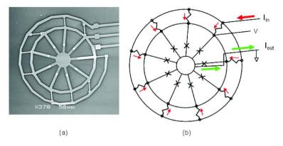
**Fig. 1** Scanning electron micrograph (a) and schematic of the device (b). In the schematic, the junctions are indicated with X's and the application of the current is shown. *Red arrows* indicate current entering the device while *green arrows* indicate current leaving the device
