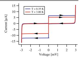
the system switches to a voltage of about 2.8 mV, the energy gap for niobium. After the current is decreased to close to zero, the system retraps back to zero voltage. The switching current is defined as the current at which the jump to the energy gap voltage occurs. As seen in the figure, lower temperatures result in larger switching currents.
