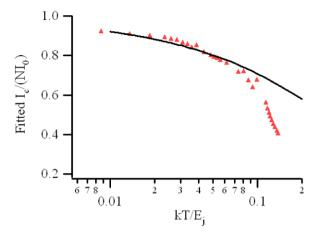
**Fig. 10** Fitted *B* (triangles) versus  $E_j/kT$ . The black line is a fit with  $\alpha = 21$ . The single-junction quantum transition temperature is indicated at  $E_j/kT$  equal to 73
